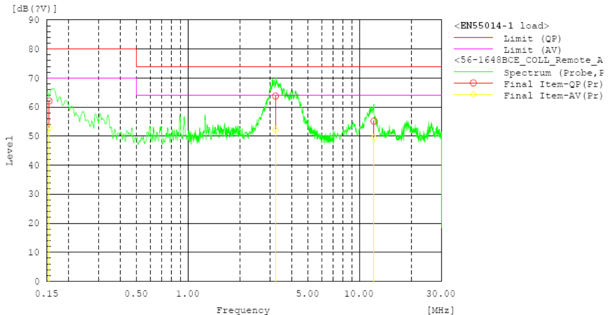
Figure 11: Spectral Diagram, Continuous Disturbance Voltage – Wired remote control cable; Operation mode A, Wired remote control cable A (Indoor side)
